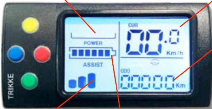
Modes: total distance, trip distance, battery voltage (V)
